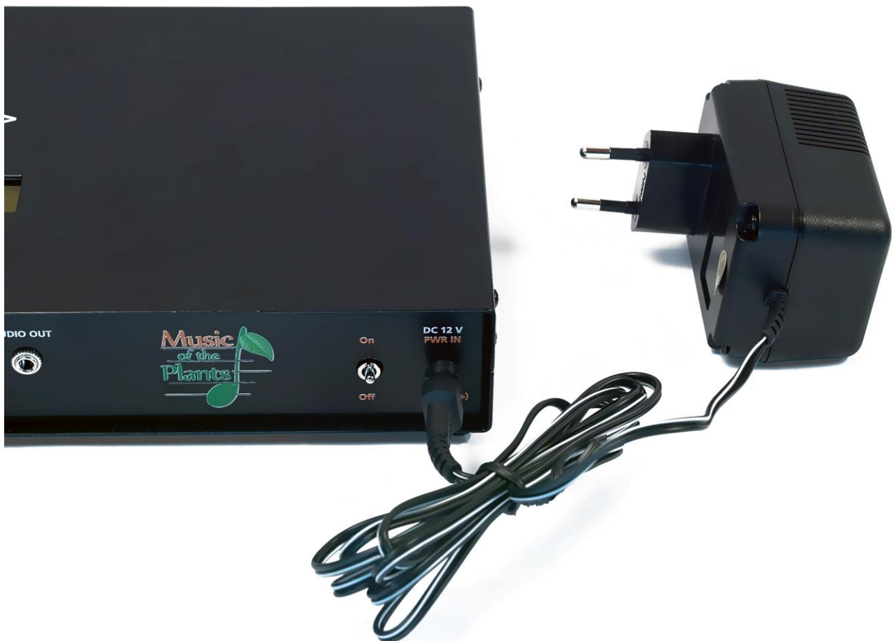
Figure 6 – View of the AC-DC transformer and its connection to the device
